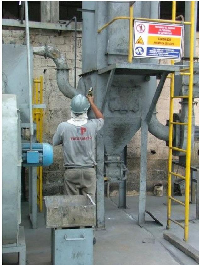
**Figure 4 : Monitoring the temperature in the baghouse**
