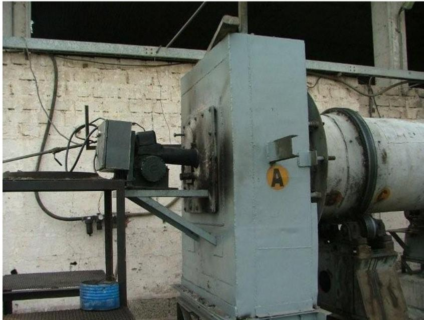
**Figure 8 : Gas lance on slag end of kiln**
